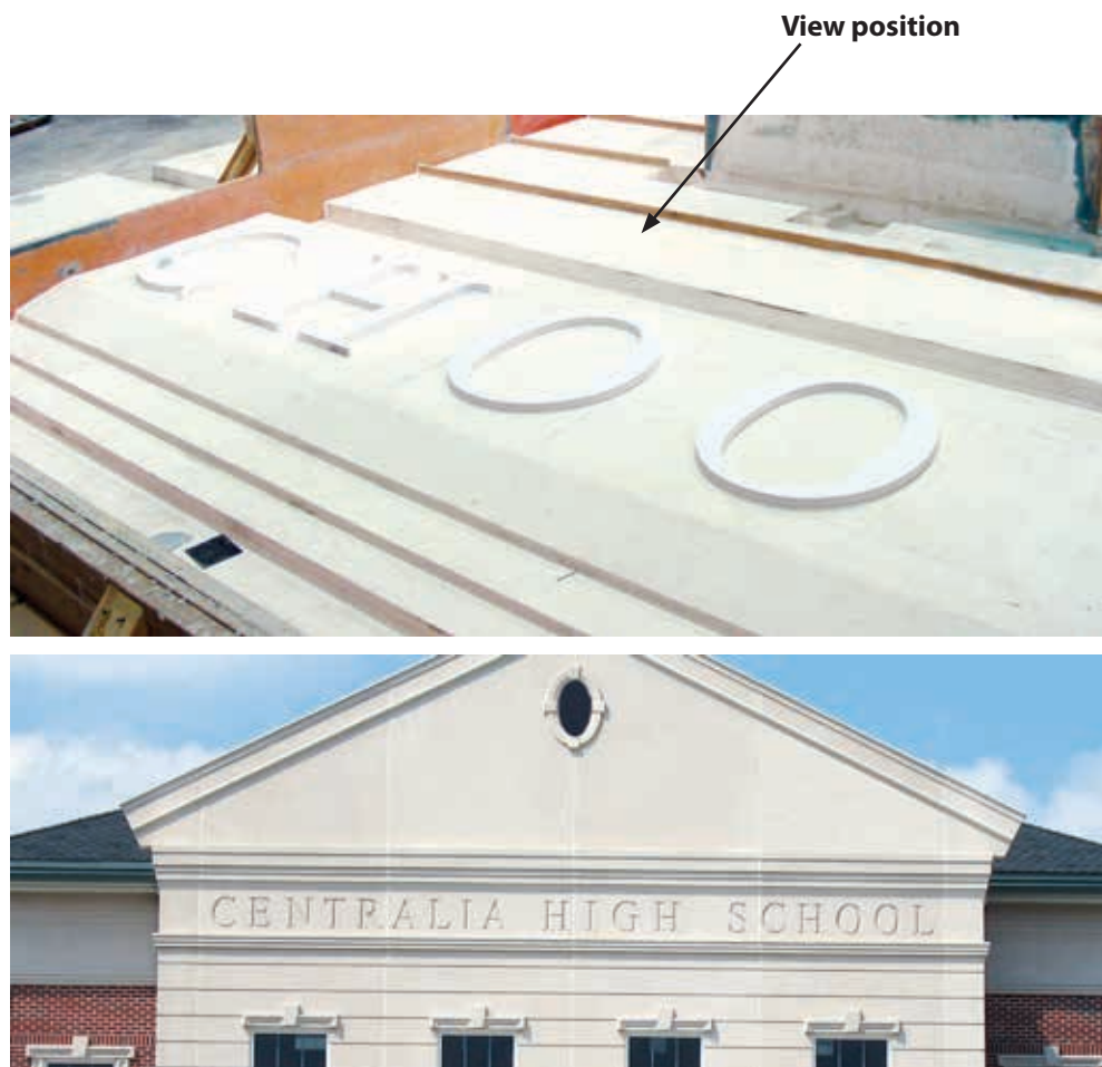
Figure 36 (a & b) Letters are reversed in the mold. Note the letter “c” that is part of the word “school”. Centralia High School, Centralia, Ill.
