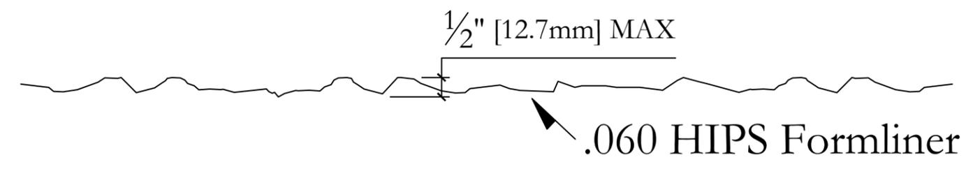
Plastic formliners MUST be stored at a temperature range of 55° to 85° Fahrenheit. Failure to do so will result in permanent distortion to these plastic formliners and will warrant them both unusable and destroyed. Therefore, AP Thermoforming will NOT assume any liability for damaged formliners caused from improper storage
