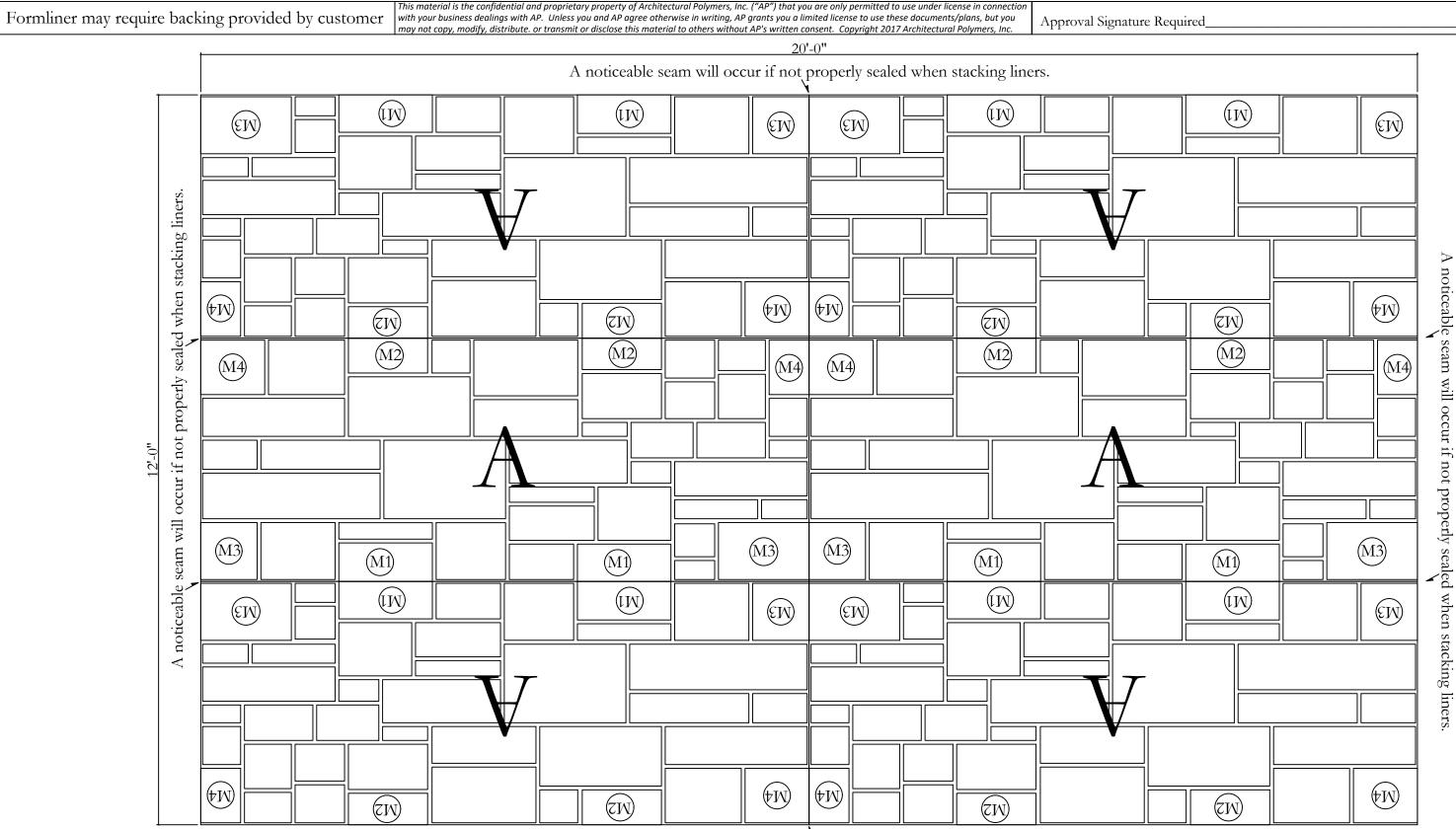
A noticeable seam will occur if not properly sealed when stacking liners.
