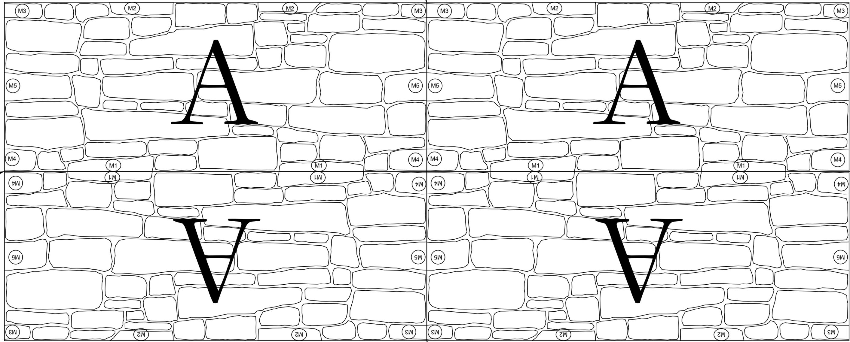
A noticeable seam will occur if not properly sealed when stacking liners.
