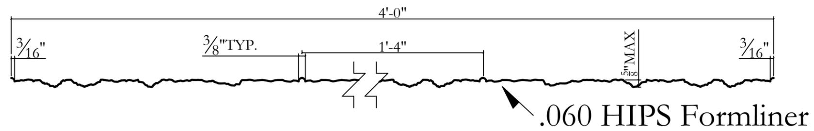
Plastic formliners MUST be stored at a temperature range of 55° to 85° Fahrenheit. Failure to do so will result in permanent distortion to these plastic formliners and will warrant them both unusable and destroyed. Therefore, AP Thermoforming will NOT assume any liability for damaged formliners caused from improper storage
