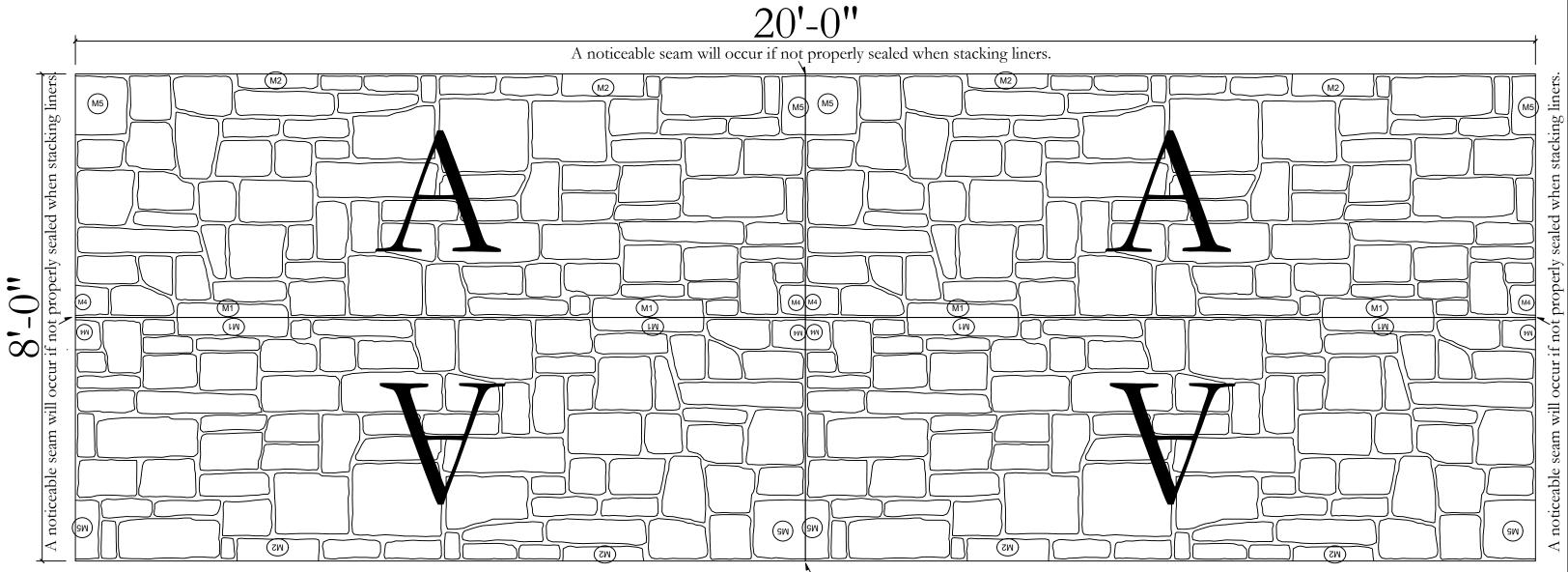
A noticeable seam will occur if not properly sealed when stacking liners.
