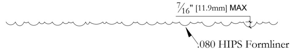
Plastic formliners MUST be stored at a temperature range of 55° to 85° Fahrenheit. Failure to do so will result in permanent distortion to these plastic formliners and will warrant them both unusable and destroyed. Therefore, AP Thermoforming will NOT assume any liability for damaged formliners caused from improper storage
