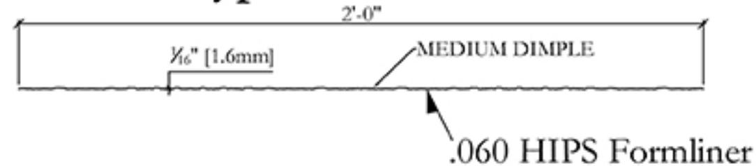
Plastic formliners MUST be stored at a temperature range of 55° to 85° Fahrenheit. Failure to do so will result in permanent distortion to these plastic formliners and will warrant them both unusable and destroyed. Therefore, AP Thermoforming will NOT assume any liability for damaged formliners caused from improper storage
