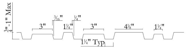
Architectural concrete surface treatment shall be obtained with Architectural Polymers® elastomeric form liner as manufactured by Architectural Polymers®. Release agent shall be approved and applied as per Architectural Polymers® recommendation. Factory bonded 3/4" plywood is also available. No substitutions will be allowed without prior written approval from the architect or engineer.
