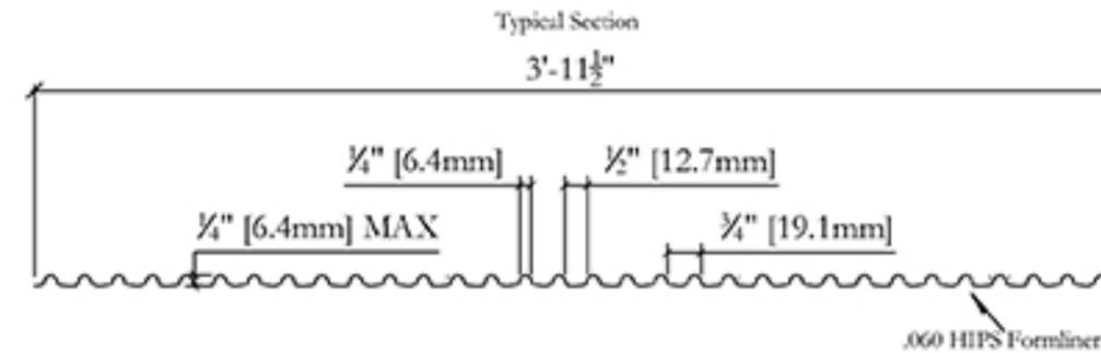
Plastic formliners MUST be stored at a temperature range of 55° to 85° Fahrenheit. Failure to do so will result in permanent distortion to these plastic formliners and will warrant them both unusable and destroyed. Therefore, AP Thermoforming will NOT assume any liability for damaged formliners caused from improper storage
