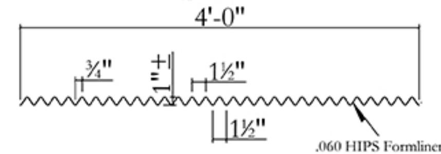
Plastic formliners MUST be stored at a temperature range of 55° to 85° Fahrenheit. Failure to do so will result in permanent distortion to these plastic formliners and will warrant them both unusable and destroyed. Therefore, AP Thermoforming will NOT assume any liability for damaged formliners caused from improper storage
