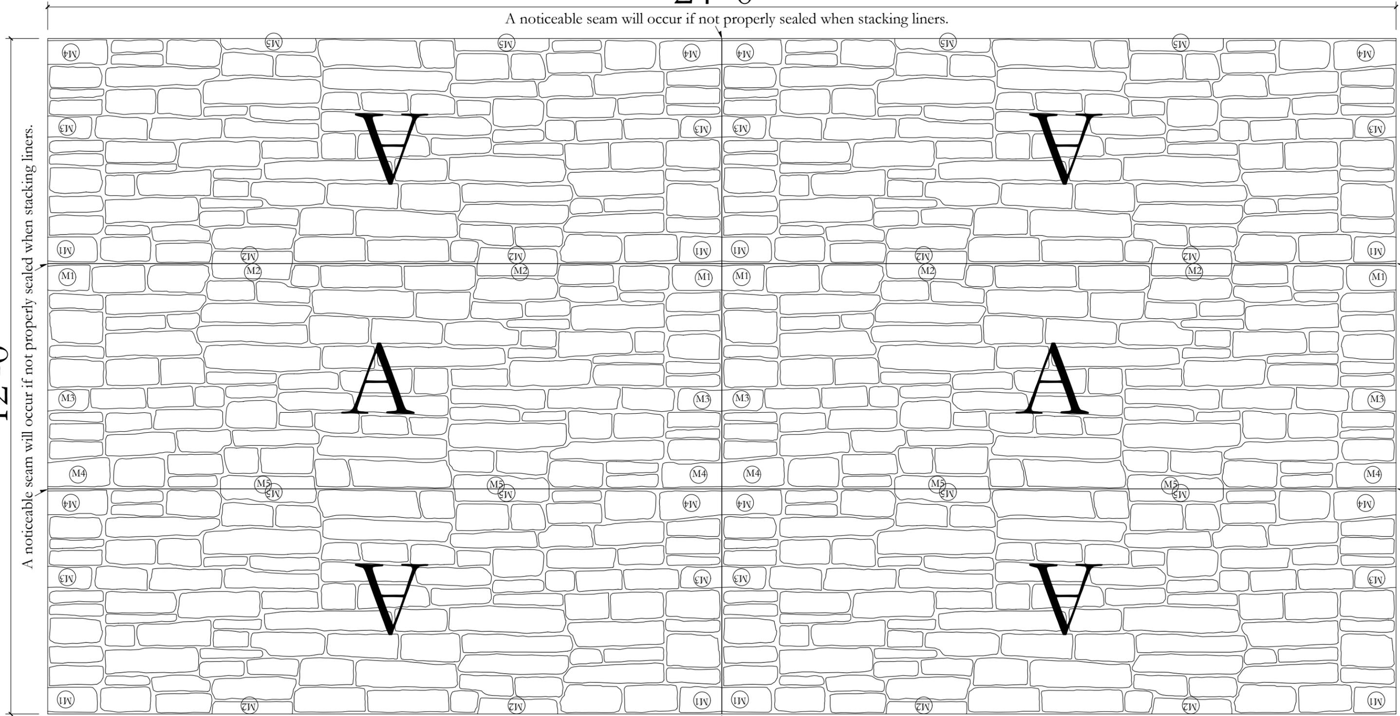
A noticeable seam will occur if not properly sealed when stacking liners.
