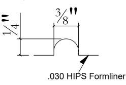
Plastic formliners MUST be stored at a temperature range of 55° to 85° Fahrenheit. Failure to do so will result in permanent distortion to these plastic formliners and will warrant them both unusable and destroyed. Therefore, AP Thermoforming will NOT assume any liability for damaged formliners caused from improper storage
