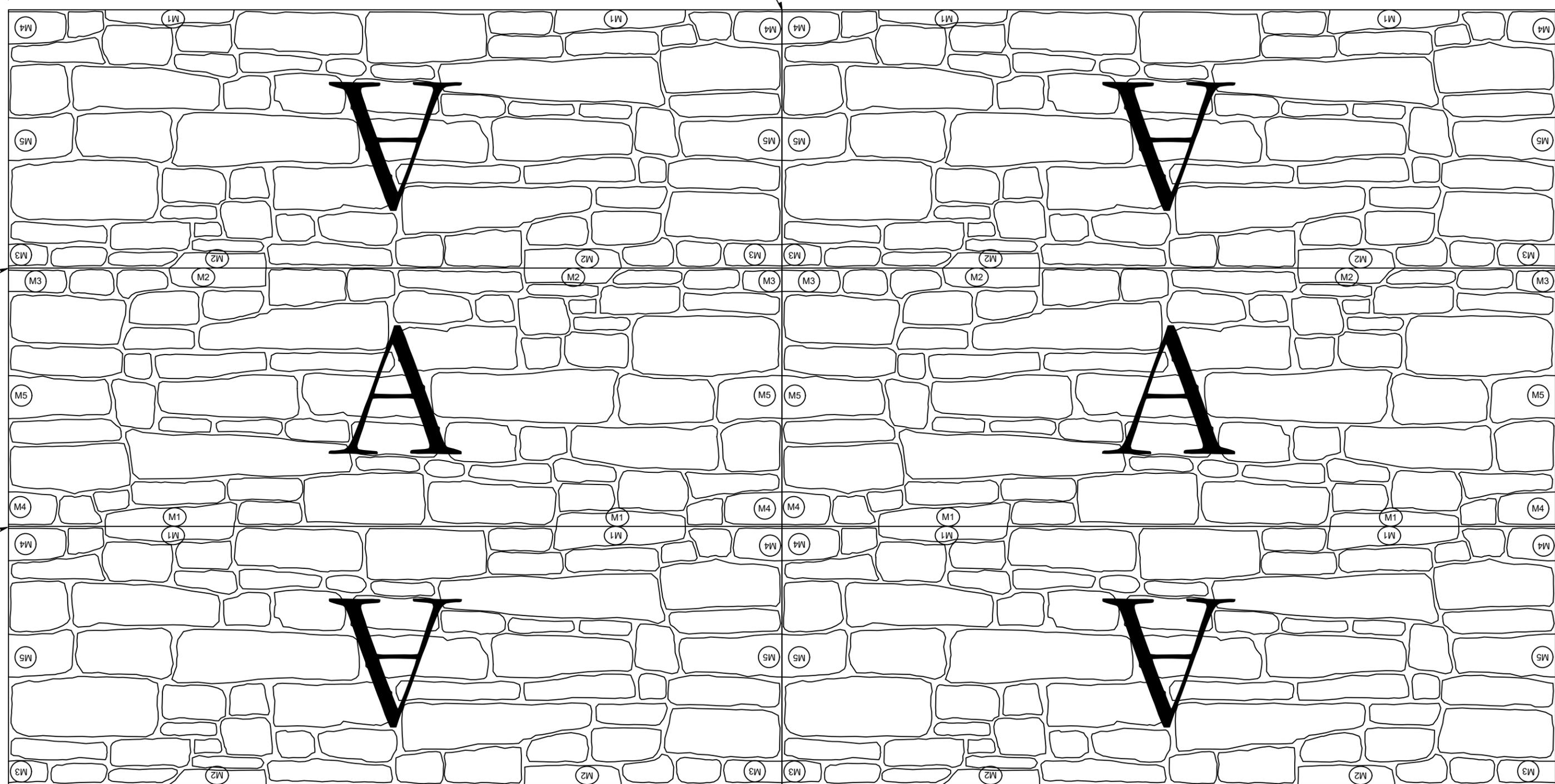
A noticeable seam will occur if not properly sealed when stacking liners.
