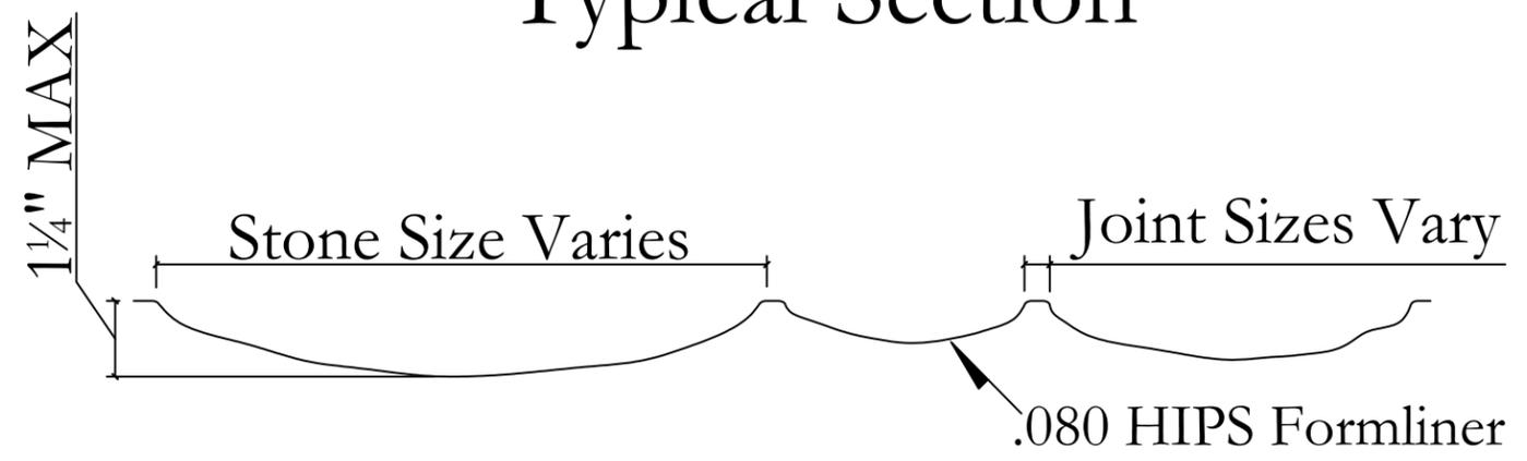
Plastic formliners MUST be stored at a temperature range of 55° to 85° Fahrenheit. Failure to do so will result in permanent distortion to these plastic formliners and will warrant them both unusable and destroyed. Therefore, AP Thermoforming will NOT assume any liability for damaged formliners caused from improper storage
