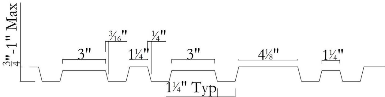
Architectural concrete surface treatment shall be obtained with Architectural Polymers® elastomeric form liner as manufactured by Architectural Polymers®. Release agent shall be approved and applied as per Architectural Polymers® recommendation. Factory bonded 3/4" plywood is also available. No substitutions will be allowed without prior written approval from the architect or engineer.
