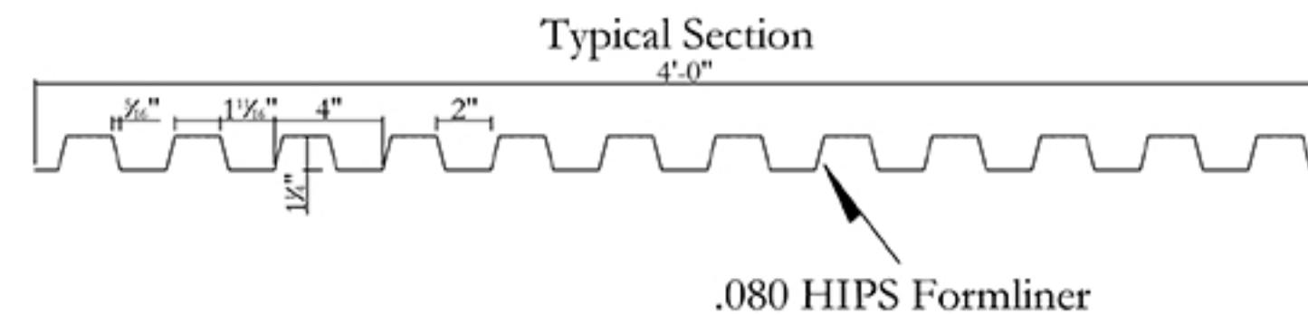
Plastic formliners MUST be stored at a temperature range of 55° to 85° Fahrenheit. Failure to do so will result in permanent distortion to these plastic formliners and will warrant them both unusable and destroyed. Therefore, AP Thermoforming will NOT assume any liability for damaged formliners caused from improper storage
